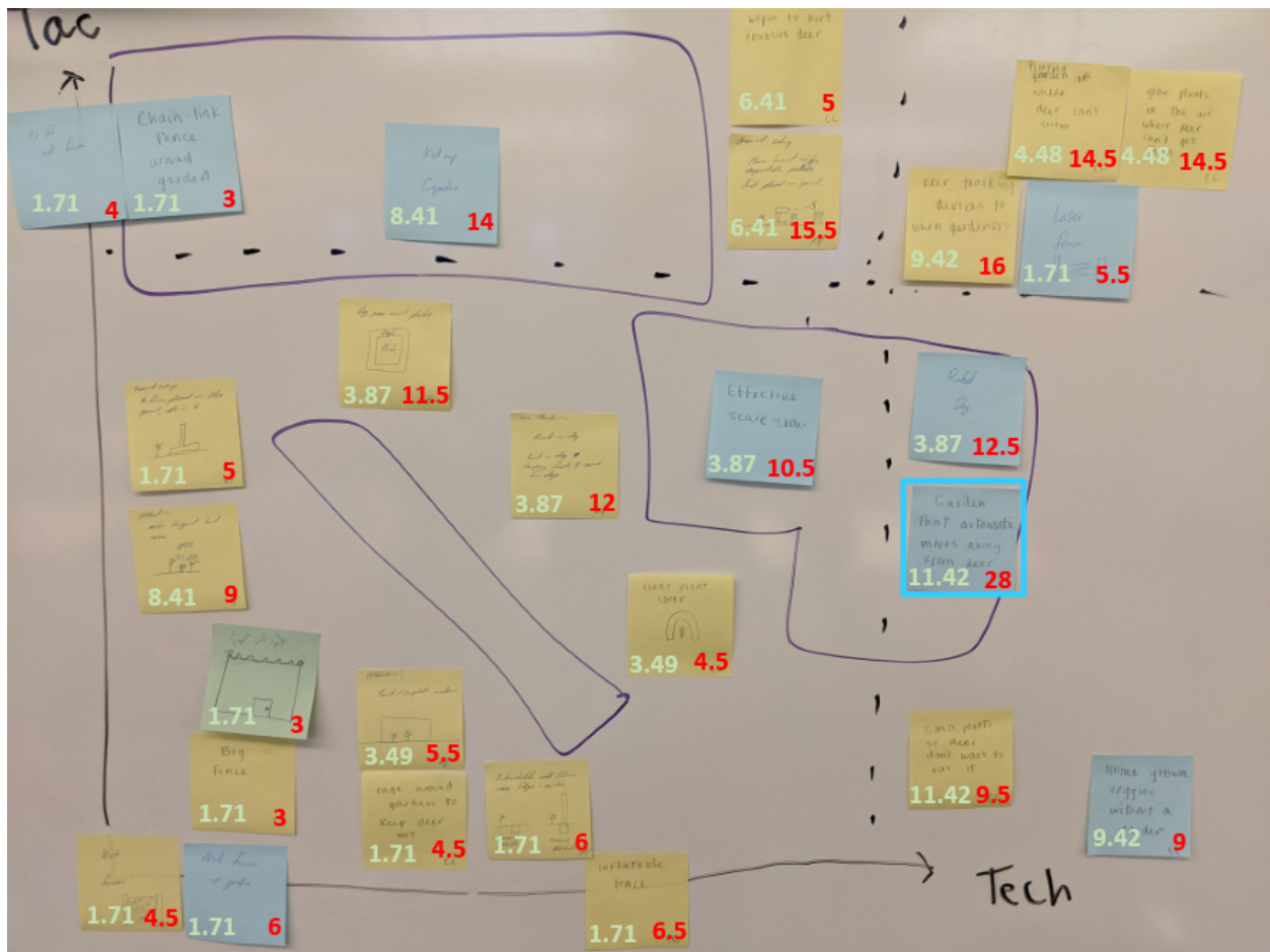
Figure 2.14: The Tech/Tac plot of Team 9 after round 2. Yellow sticky notes represent round 1 concepts, while blue or green sticky notes represent round 2 concepts. Novelty (in red) and allocated variety (in green) scores for each concept have been superimposed over each concept. The highlighted concept is a high-scoring round 2 concept that was found in an empty space identified by the team
